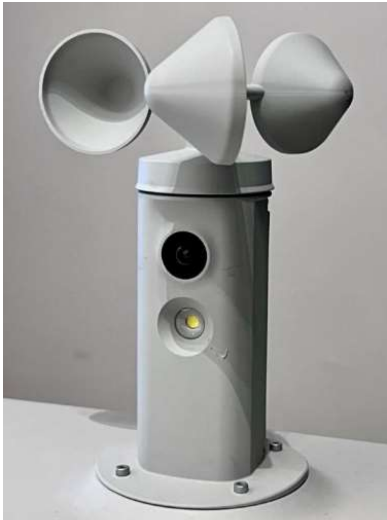
Figure 2-4 Wind speed gauge
