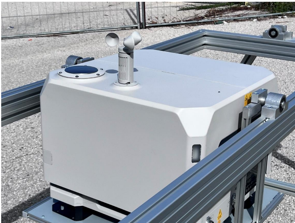
Figure 1-4 UAS recharging station installed in the tilting mechanism – side view
