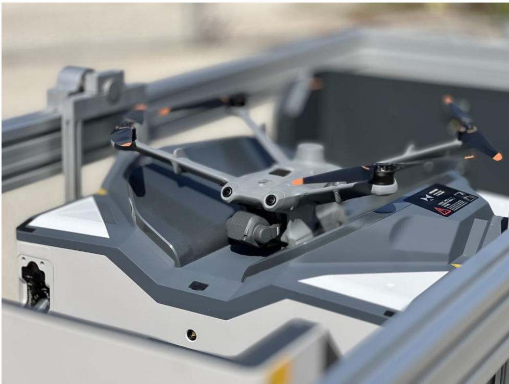
Figure 1-9 Detail of the UAS placed in the tilting mechanism
