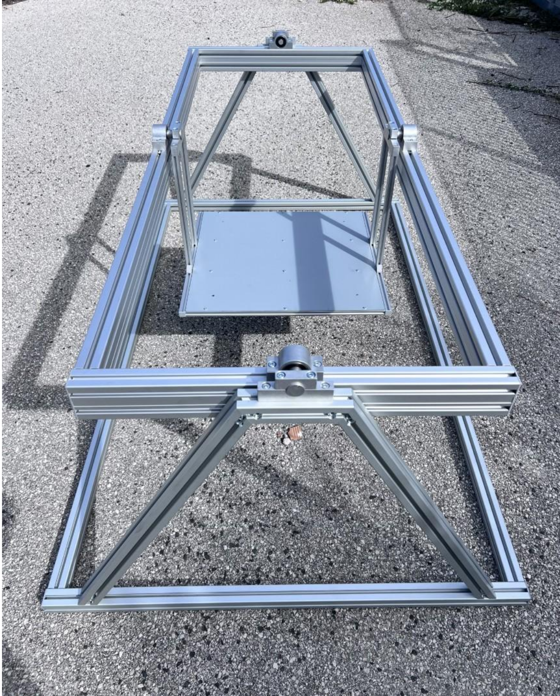
Figure 1-2 The tilting mechanism of the vessel version
