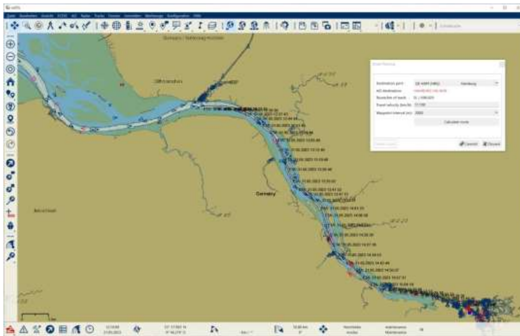
Figure 39- Example of route planning on the ECDIS/ VTS and PPU user interface
