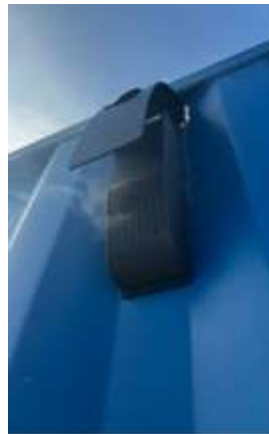
Figure 23- Sensor unit for early fire detection inside containers
